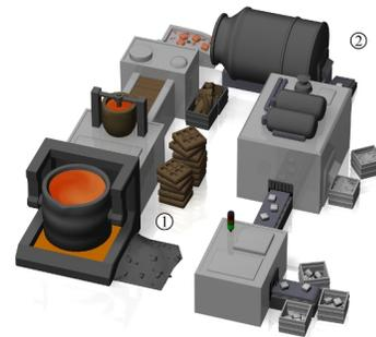
Fig. 1. Foundry process work flow showing the different phases castings have to pass through. More accurately, in 1 it is performed the metal melting step, and in 2 it is performed the casting preparation and separation step.
