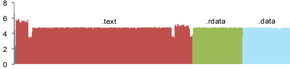
Fig. 2. Entropy profile of the analysed sample, that represents the randomness of the file in a fine-grained style.
